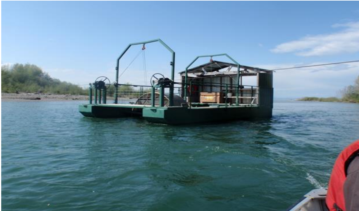
Figure 2. Top Elwha River 8' rotary screw trap fishing at Rkm 0.3 during the pre-dam and post-dam removal periods and bottom 5' rotary screw trap used during the dam removal period.
